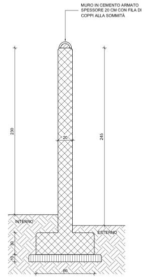
DETTAGLIO MURO IN C.A. SCALA 1:20
